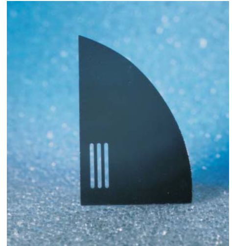
Fig. 1: Part of a silicon wafer with laser cut structures
