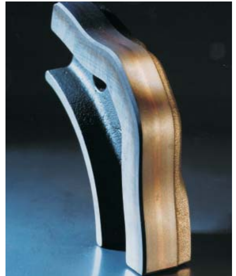
Fig. 3: Laser beam hardened curved gripper edge, hardness 800 HV 0.05, optional hardening depth 0.1
