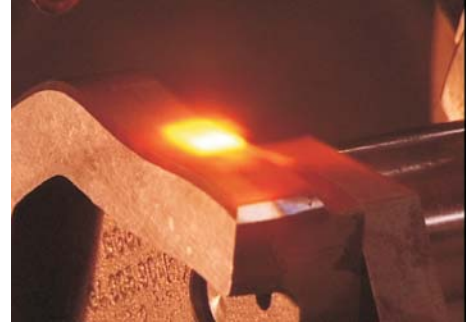
Fig. 2: Hardening of a curved gripper edge with high power diode laser
