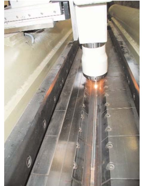
Fig. 1: Welding of a Cr-Ni-steel tank with 2,5 kW diode laser
