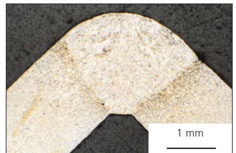
Fig. 4: Welding of steel tanks without filler
