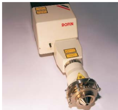
Fig. 6: Cladding with diode laser and cyclon powder feeder head
