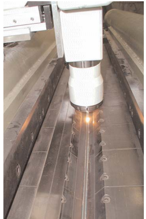
Fig. 2: Welding of large sheet metal components by a 2.5 kW HPDL
