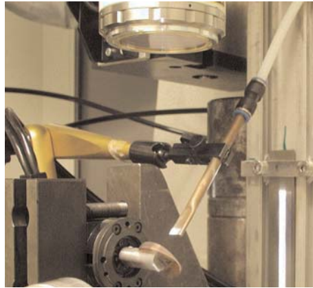
Fig. 8: Lab construction - scanner system for 2.5 kW high power diode laser, - maximum with a homogeneous power splitting 100 mm
