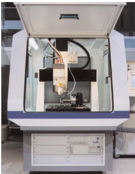
Fig. 1: Laser hardening plant with integrated high power diode laser (HPDL)
