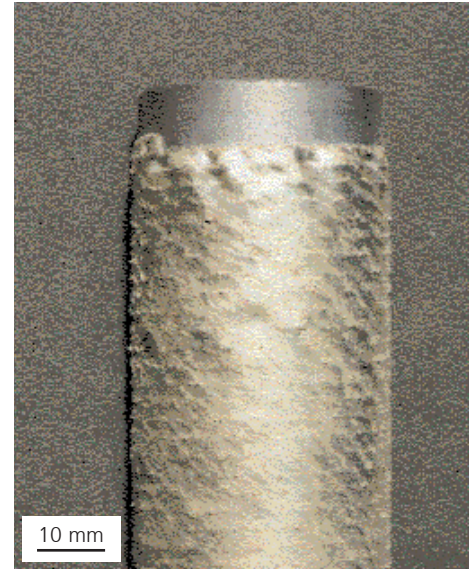
Fig. 10: Cold work steel 90MnCrV8 (O2) crack-free coated with NiCrBSi alloy Deloro 60
