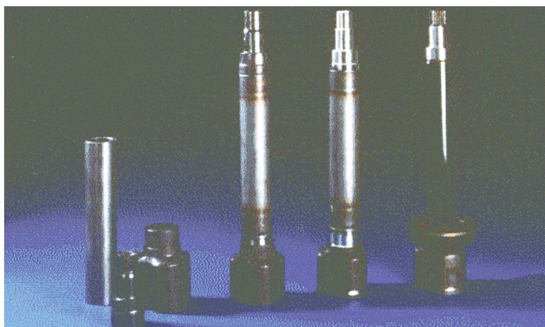
Fig. 6: Induction assisted laser beam welding in production in the automotive industry: Welding of drive shafts at Ford Motor Co., Cologne, Germany
