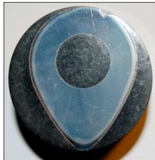
(c) camshaft lobe showing selective hardened outer layer of lobe
