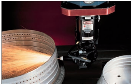
Figure 2. LAI International uses trepanning laser drilling process to produce hundreds of precision shaped cooling holes in aerospace combustor components.
