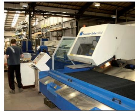
up to 20 mm thick mild steel, 15 mm stainless steel and 10 mm aluminium. Typical Trumpf innovation is applied in the form of an additional Y-axis integrated in the motion unit. Unlike the standard Y axis, it does not move the complete motion unit, only the cutting head. The intelligent application of a double axis greatly increases the dynamics and reaction time of the machine and, particularly on small part geometry, processing time can be reduced by up to 30%.
