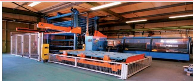
Like Stevens & Carlotti's previous Platino/TowerServer combination, the CompactServer equipped machine also runs under ‘lights out’ conditions if required.
